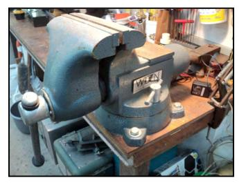
ABOVE: The vise on the left is designed to hold round objects. The vise will firmly hold a round item in either a horizontal or vertical position. And when you really need to hold something from moving the vise on the right is the ultimate bench vise. This vise has wide 6-inch jaws, 360 degrees of swivel adjustment and a small flat surface plate if a hammer is needed to straighten an item. This vise is bolted to the workbench with ½ inch bolts.
