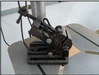
ABOVE: These sturdy drill press vises have long slots to enable them to be firmly attached to the drill press table. The vise on the right is fully adjustable from 0 to 90 degrees.
