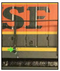
So what might the prototype do when a handrail breaks off from the frame? Drill a new hole and insert a new bolt.
